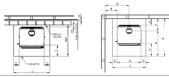
**Above: Non combustible wall clearances.** Brick lining. From the floor to within 25mm of ceiling. Leave air vents at the bottom to allow airflow in the cavity. If Yunca flue mounted shield is fitted, brickwork may be 1200mm high as long as all vertical joints in top and bottom of brickwork are left out to allow airflow when brickwork is capped.
